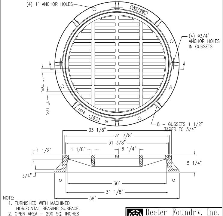
MATERIAL: CAST GRAY IRON ASTM A-48, CLASS 35B
