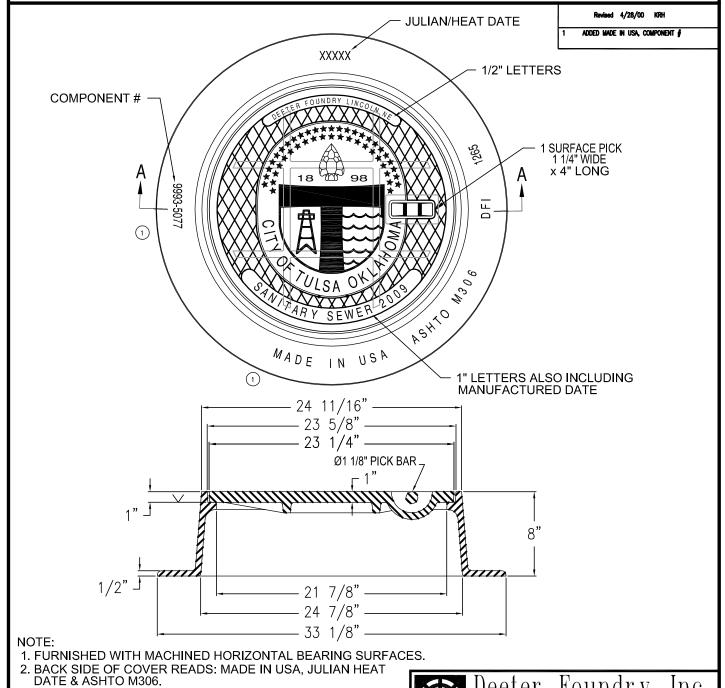
MATERIAL: CAST GRAY IRON ASTM A-48, CLASS 35B FINISH: NO PAINT WEIGHT: FRAME 160 LBS.
